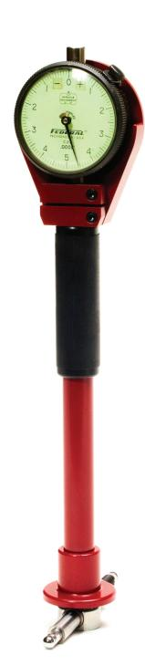
The Internal Pitch Diameter gage is a specific "single dimension" gage utilizing the unique features of the bore gage. It is adapted solely to check the internal diameter of gears and splines but can be used to check any internal dimension where centralization is not necessary.
