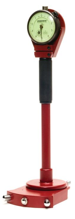
Bore gages are comparator instruments designed to evaluate conditions of internal diameters. Readings on the dial indicator can be interpreted as limited fluctuations similar to "go" and "not go" readings for quick inspections, or they can be easily converted to a dimensional value.
