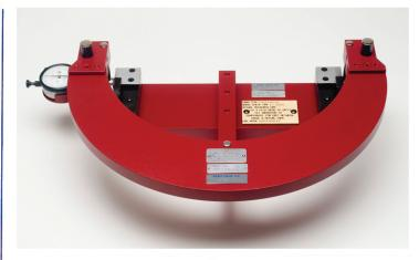
This large diameter gage is specifically designed to encircle the part being gaged. The advantages of this design are obvious as central obstructions or long part units are encountered.
