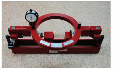
A single dimension gage constructed to allow for central interference caused by part obstruction or a fixture set up. The frame is selected by part print to allow clearance completely around the interference but maintain accurate rigid centerline diameter gaging.
